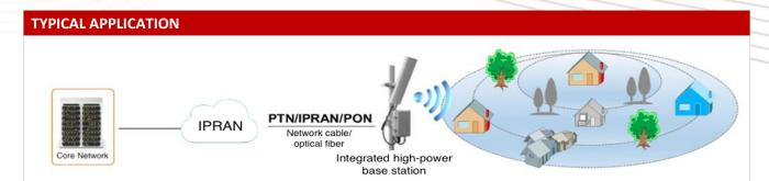
In rural and suburban areas, the wireless network coverage is relatively wide, but the users are less fixed than the fixed ones. By deploying LTE integrated high-power base stations in a town or natural village, the signal coverage in a small area can be achieved, reaching low Investment in rural 4G wireless access.
