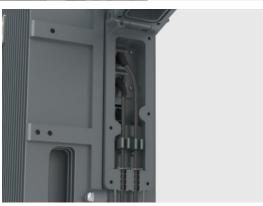
**Step 1:** Open the chassis on the right side of the RU4460 and connect to the SFP optical module.
