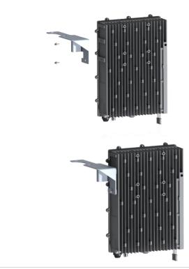
Using a T5 wrench, secure the BBU Mounting bracket to the left side of the device with M6\*12 screws
