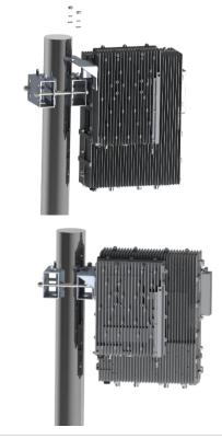
Hang the BBU on the mounting bracket and secure with the M10 nut
